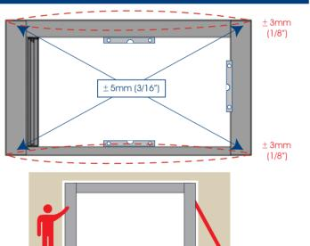
PROVIDE TEMPORARY SUPPORTS TO BOTH JAMBS TO PREVENT SCREEN FALLING
